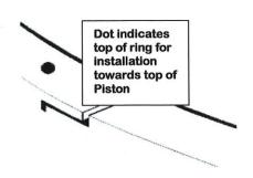
PLEASE NOTE: Do not assemble engine before checking all piston ring end gaps.
