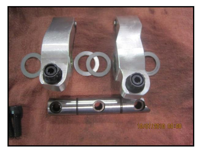
WHEN SETTING THE ROCKER ARM SHAFT ASSEMBLY ON TO THE PEDISTAL, BE CAREFUL NOT TO DAMAGE THE (4) THRUST SHIMS.
