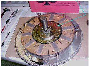
8. Align top disc splines w/bottom disc splines. Install pressure plate. Line up ink marks with center plate and flywheel. Torque nuts to 30 ft lbs, use blue Loctite 242.
