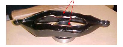
AFTER INSTALLATION OF TRANSMISSION, TIGHTEN ALL BELL HOUSING BOLTS. <u>DO NOT INSTALL SLAVE CYLINDER</u>. INSERT FINGER IN SLAVE CYLINDER HOLE MAKING SURE THROW OUT BEARING ARM HAS A MINIMUM OF 1/4" MOVEMENT FRONT TO BACK.
