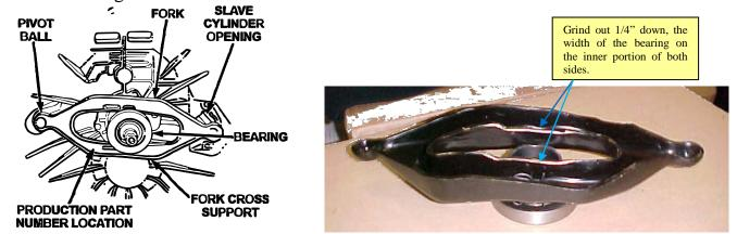
AFTER INSTALLATION OF TRANSMISSION, TIGHTEN ALL BELL HOUSING BOLTS. <u>DO NOT</u> <u>INSTALL SLAVE CYLINDER</u>. INSERT FINGER IN SLAVE CYLINDER HOLE MAKING SURE THROW OUT BEARING ARM HAS A MINIMUM OF ¼" MOVEMENT FRONT TO BACK.
