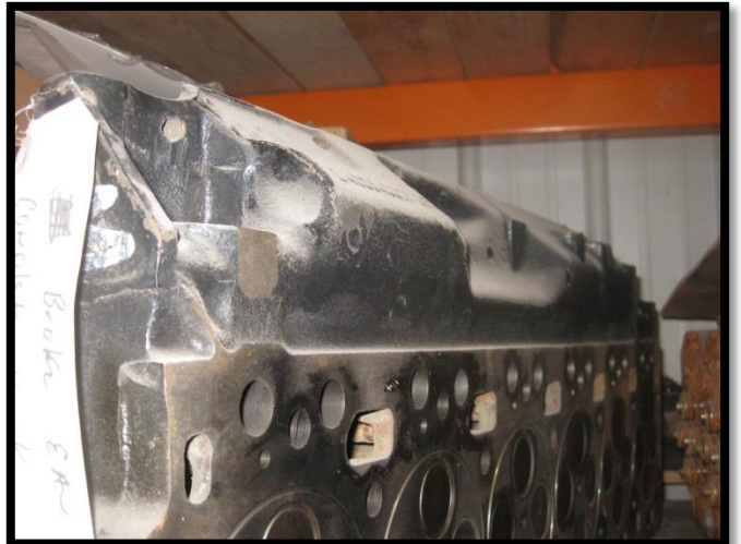
Above & Below: 5.9L, 24V, ISB, 1998.5-2002. Intake has big "lump" in the center and back side has more of a sharp edge transition.
