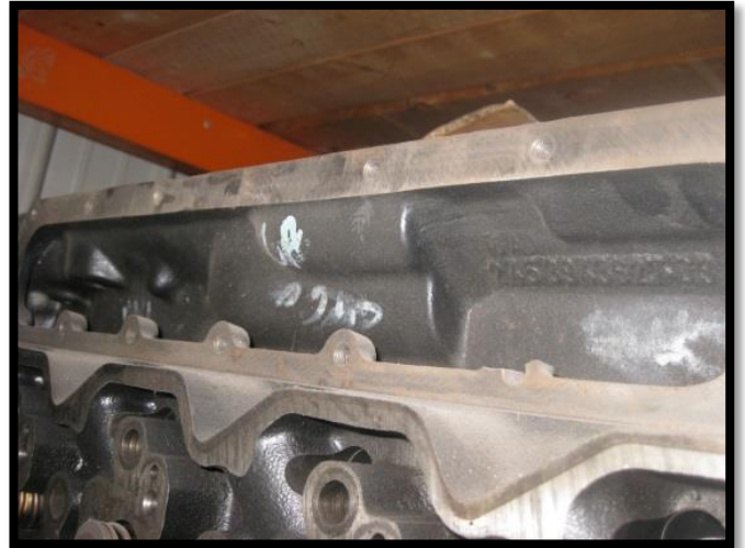
Above & Below: 5.9L, 24V, ISB, 1998.5-2002. Intake has big "lump" in the center and back side has more of a sharp edge transition.
